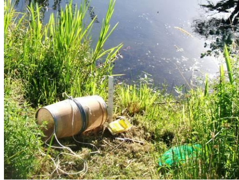
Photo 19. Gee Minnow trap with pantyhose covering.
